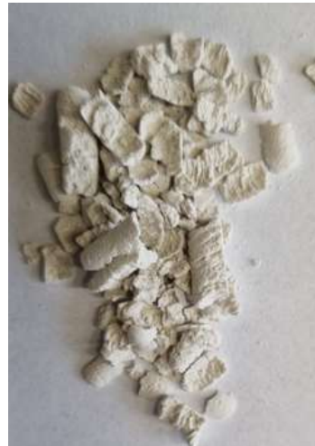
Fig.7 Influence of the screw and rotor speed and die geometry L/D = 5 mm / 4 mm on the product quality.
