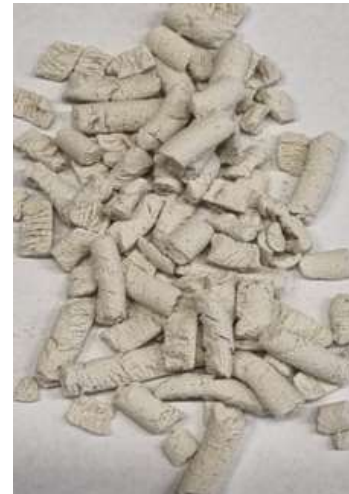
Fig.8 Influence of the screw and rotor speed and die geometry L/D = 9 mm / 4 mm on the product quality.
