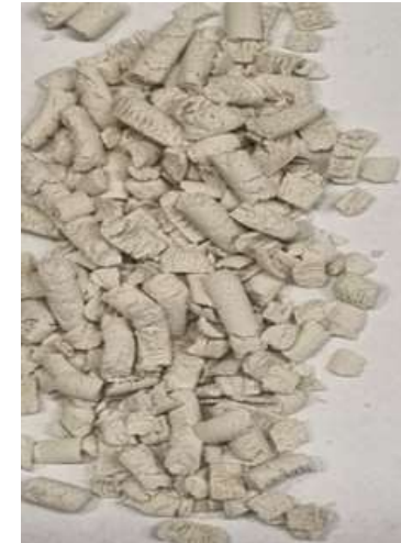
Fig.8 Influence of the screw and rotor speed and die geometry L/D = 9 mm / 4 mm on the product quality.
