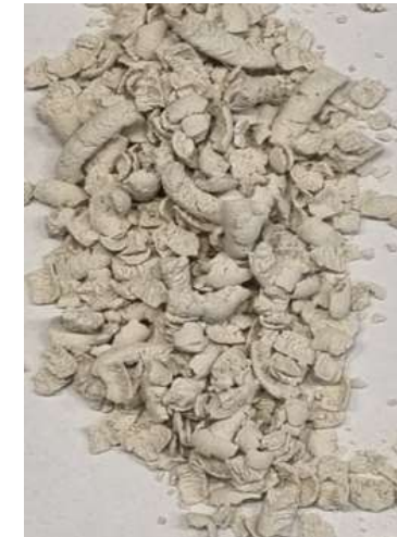
Fig.7 Influence of the screw and rotor speed and die geometry L/D = 5 mm / 4 mm on the product quality.
