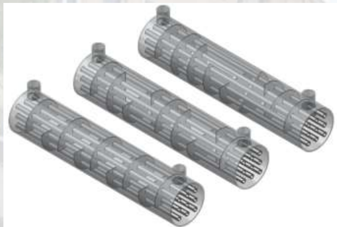
rotated segment baffles
