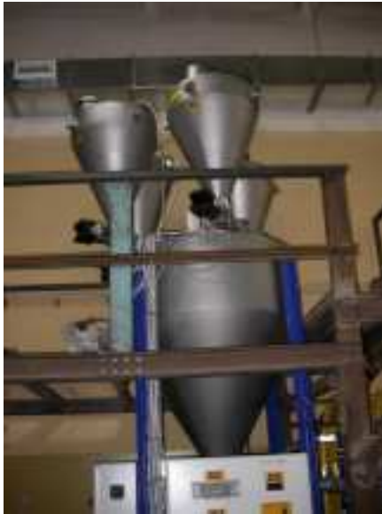
4 dispensers and a mixing unit
