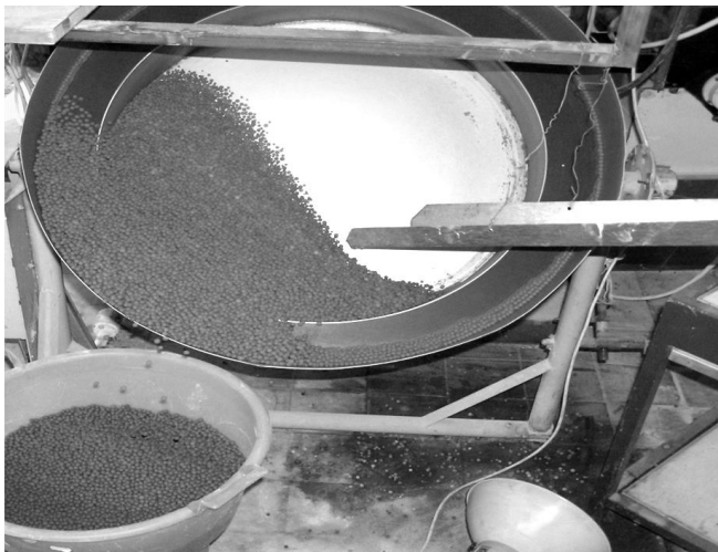
Coating of the granules by the cement.
